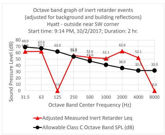
Figure 9. Octave band plot of adjusted measured inert retarder  $L_{eq}$  from 9:14 PM to 11:14 PM, October 2, 2017, outside Hyatt Place hotel and allowable nighttime levels from Class C land emitted to Class A land.
