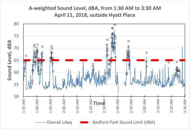
Figure 10. Time history of A-weighted 10-second equivalent sound levels (dBA) from 1:30 AM to 3:30 AM, April 11, 2018, outside Hyatt Place hotel and non-quiet hour limit in Bedford Park ordinance. (Periods dominated by inert retarder noise are marked by circles.)
