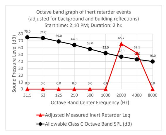
Figure 6. Octave band sound pressure levels for adjusted measured inert retarder  $L_{eq}$  for Period 3, 2:10 PM to 4:10 PM, April 11, 2018, outside Hyatt Place hotel and allowable daytime levels from Class C land emitted to Class A land,
