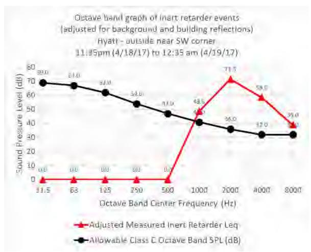
Figure 8. Octave band plot of adjusted measured inert retarder  $L_{eq}$  from 11:35 PM to 12:25 AM, April 18-19, 2017, outside Hyatt Place hotel and allowable nighttime levels from Class C land emitted to Class A land.
