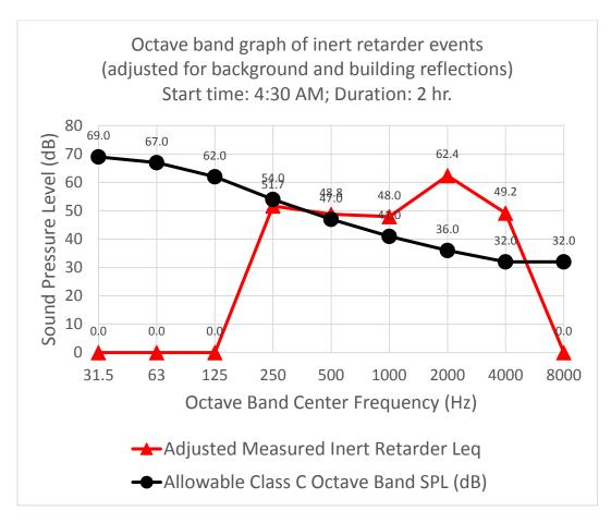
Figure 5. Octave band sound pressure levels for adjusted measured inert retarder  $L_{eq}$  for Period 2, 4:30 AM to 6:30 AM, April 11, 2018, outside Hyatt Place hotel and allowable nighttime levels from Class C land emitted to Class A land.
