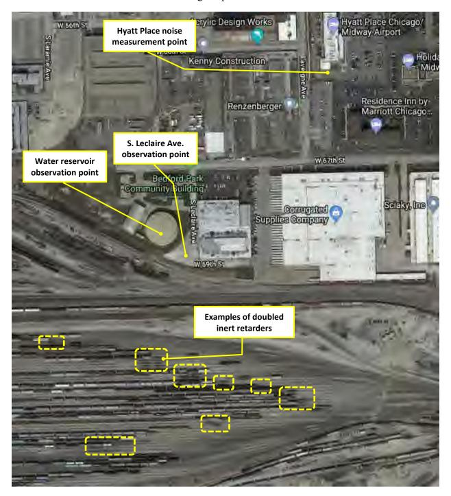
Figure 3. Hyatt Place noise measurement location, observation points and some visible inert retarders in dashed yellow boxes (others are not visible, as they are under the rightmost cars on the other tracks). (Google Maps)
